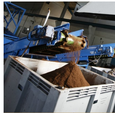
Capsule recycling: separating the coffee grounds from the aluminium
